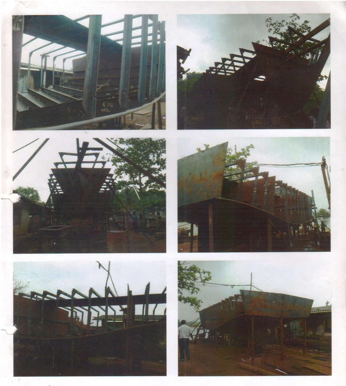
Fig.1.(a) Construction of keel of training vessel "Ocean Queen" at workshop
